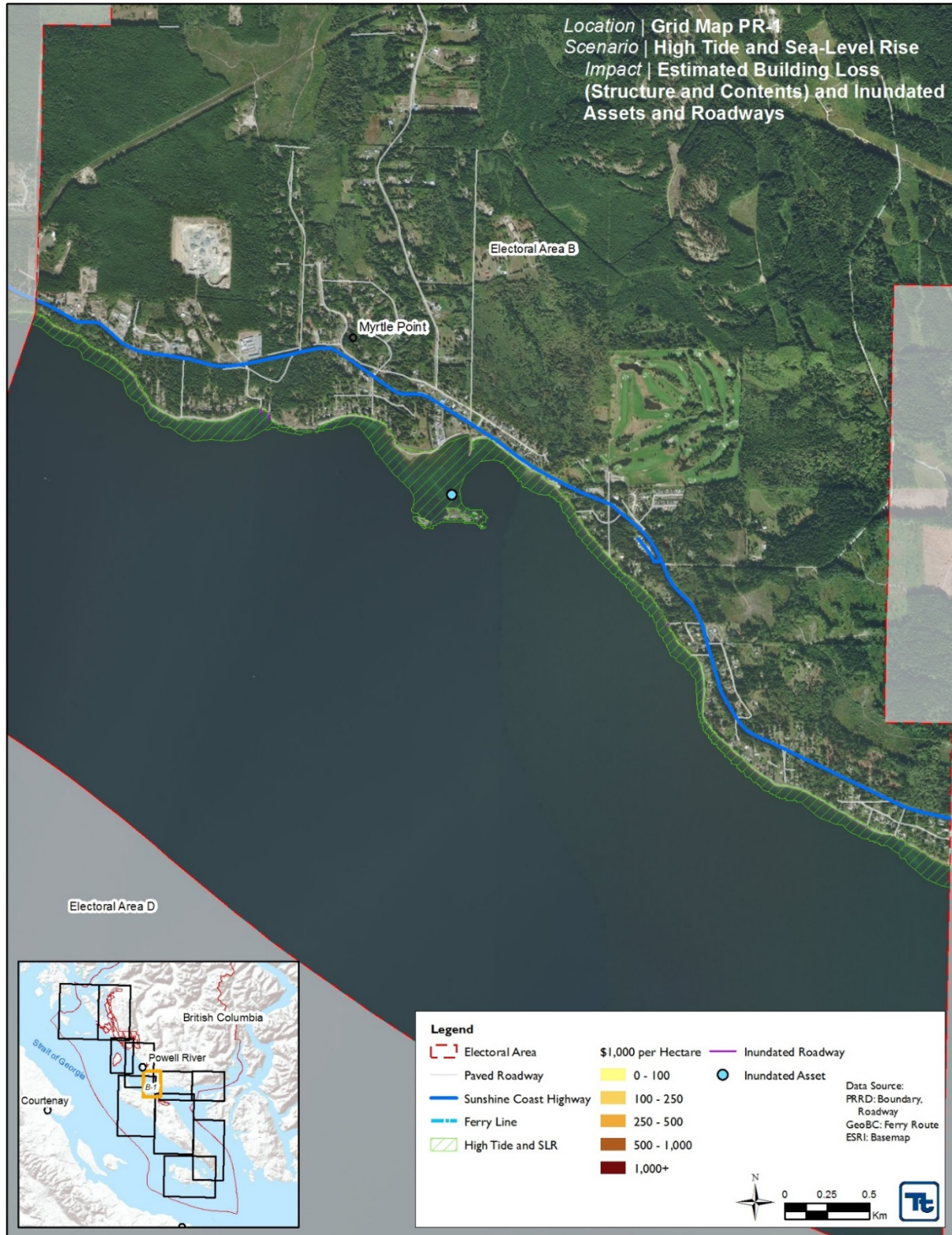
Figure 27. Grid Map B-1 with Estimated Building Exposure (Structure and Contents) and Inundated Assets and Roadways for the High Tide and Sea-Level Rise Scenario
