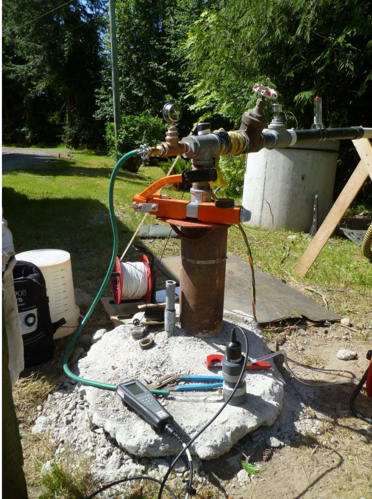
Photo 3: Wellhead arrangement for pumping test and flow through cell for water quality measurements.
