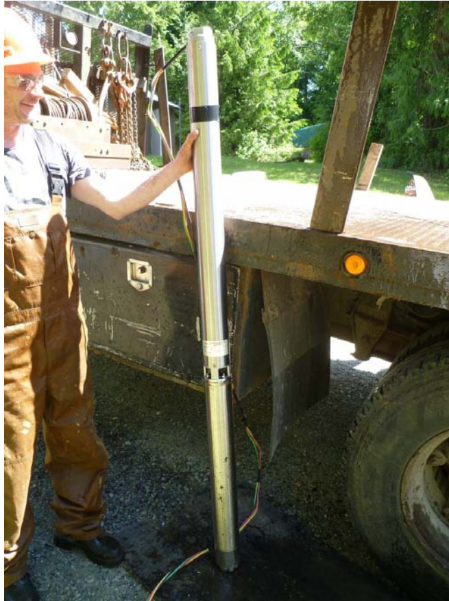
Photo 1: 7.5 hp 3 phase test pump
