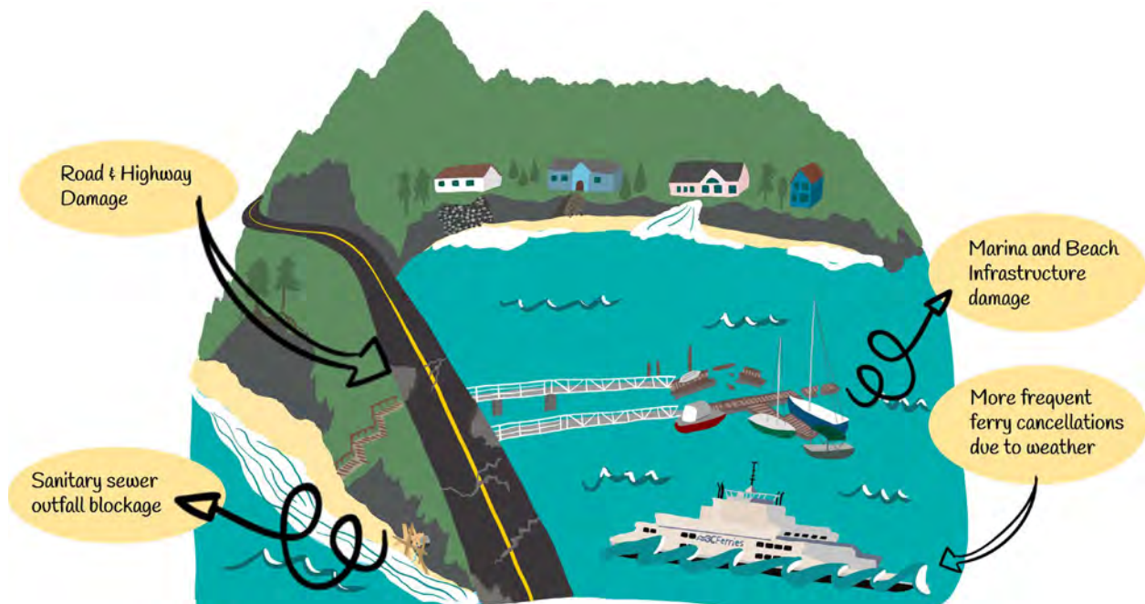
Figure 5-1: Infrastructure damage and destruction.
